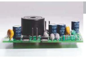
Acoustic device to indicate wrong installation (buzzer).
