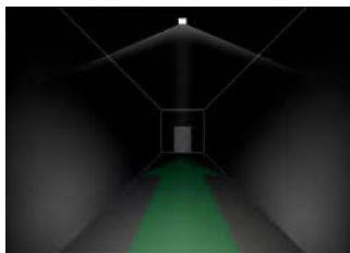
Escape route illumination with symmetric optics
