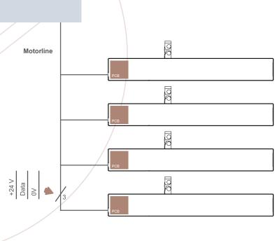
All WindowMaster MotorLink<sup>®</sup> field bus solutions support data objects giving options for position control with different speed and priority as well as feedback of actual position and detailed status of the connected actuators.
