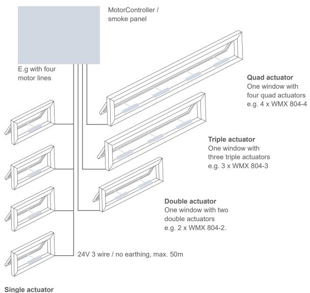
One window with one single actuator e.g. 1 x WMX 804-1. Up to four windows each with one actuator e.g. 4 x WMX 804-1 can be connected.)
