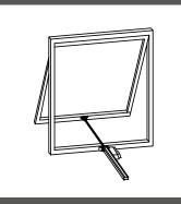
On top hinged window without windowsill with front fixing through end bracket part No. 40234E
