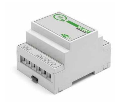
This Control unit offers a direct WI-FI access point for PCs, smartphones and tablets, or can be connected with the LAN installed in the building. BMSline actuators and sensors are connected by means of a special bus line (Modbus RTU). The web based (HTML5) user-interface is accessible in three different levels:
