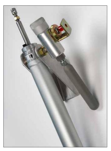
The valves pierce the CO<sub>2</sub> cartridge in response to a thermal or electric (when the pyrotechnic device is installed) signal. The CO<sub>2</sub> flows into the cylinder and causes the window opening.
