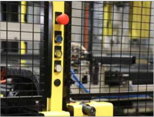
Post, push buttons The post (50x50 or 70x70) is prepared for up to 5 push buttons (not included). It is also equipped with a cover plate that doubles up as a guard against accidental activation.
