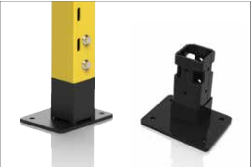
Foot 70x70 mm The 70x70 post includes a black powder coated foot. It can be fitted at four different angles. Top plug and expansion bolt for floor fixing included. Floor gap 100 mm.
