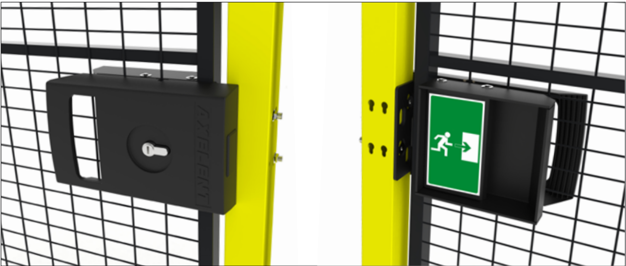
X-It Panic lock A lock with cylinder can be used as an emergency exit and means of escape where maintenance access is required. Doors with panic lock can always be opened from the inside, even when locked by key from the exterior.
