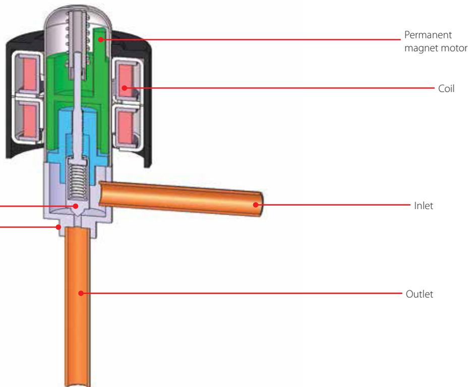
Cross section diagram of ETS 6 series
