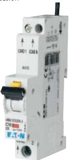
**Electronic Combined RCD/MCB Devices eRBM-AU, 1MU****1+N-pole****Conditionally surge current-proof 250 A, sensitive to residual pulsating DC, type A**
